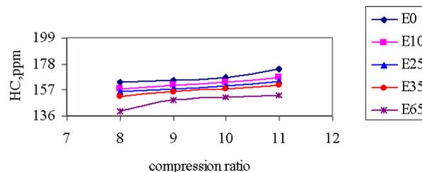
**Figure 13.** Variation of hydrocarbon emissions with compression ratio.
