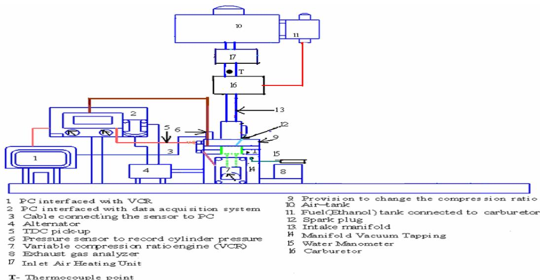
**Figure 1.** Experimental test rig with necessary instrumentation.
