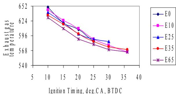
**Figure 11.** Variation of exhaust gas temperature with ignition timing at the compression ratio of 11:1.
