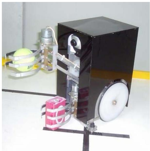
**Figure 6.** Manufactured differential drive robot (Case III)
