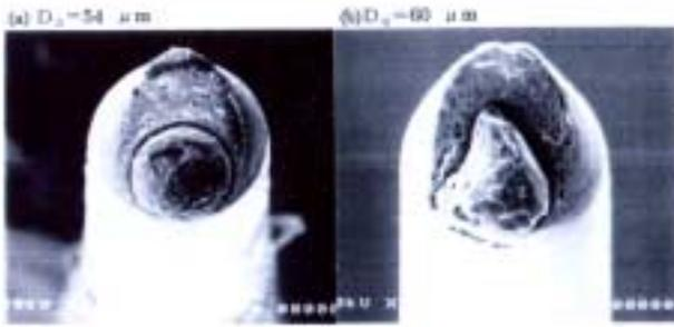
**Figure 3.** Wire breakage due to an inclusion: a)  $D_0 = 54 \mu\text{m}$  b)  $D_0 = 60 \mu\text{m}$  [1].
