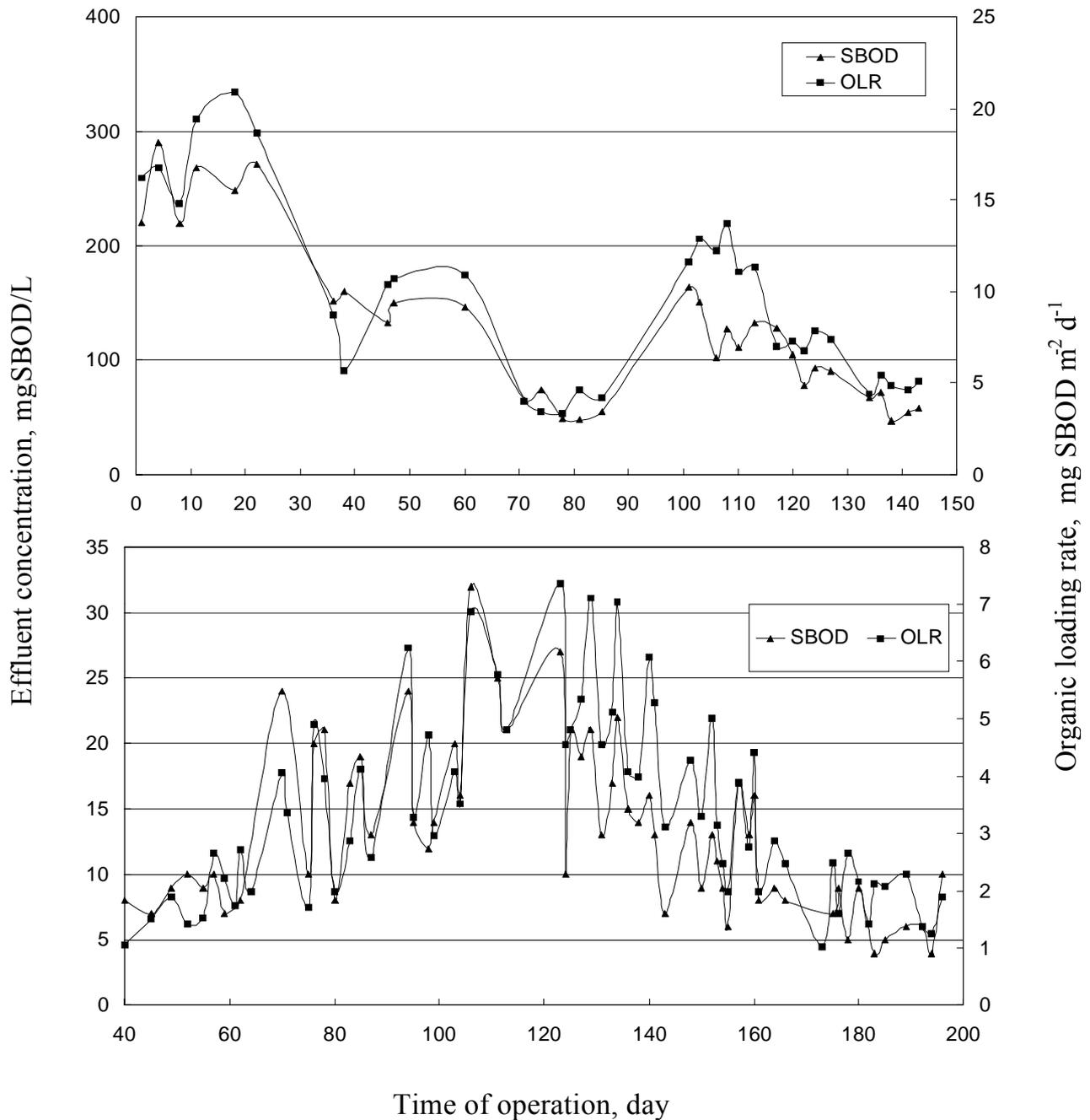
**Figure 3.** Effluent concentration of the RBC reactor at different organic loading rates(top: industrial, bottom: municipal).
