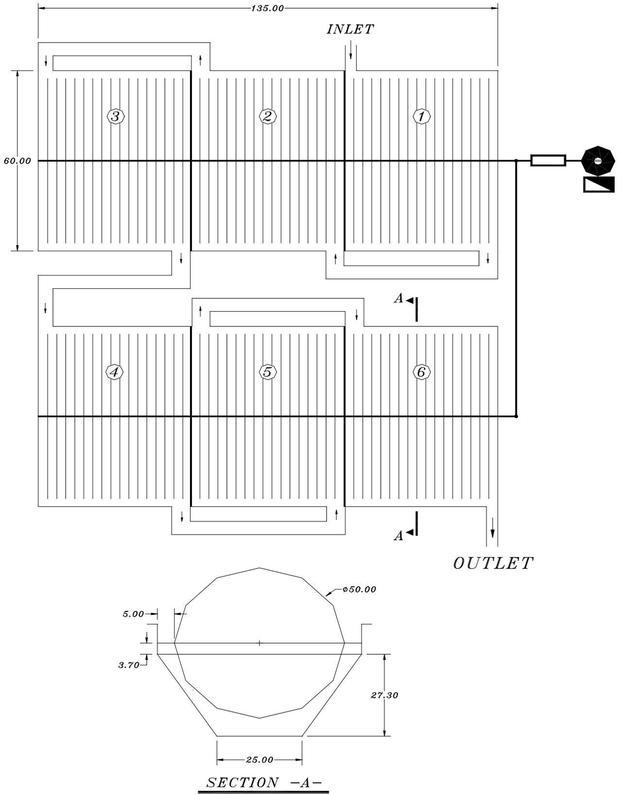
**Figure 1.** Schematic diagram of rotating biological contactor.
