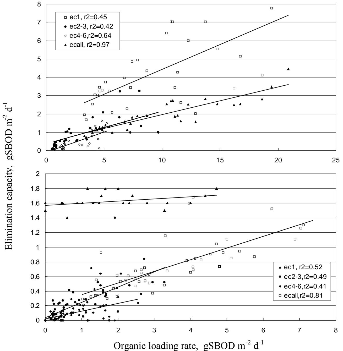
**Figure 5.** Elimination capacity of the RBC reactor at different organic loading rates(top: industrial, bottom: municipal).
