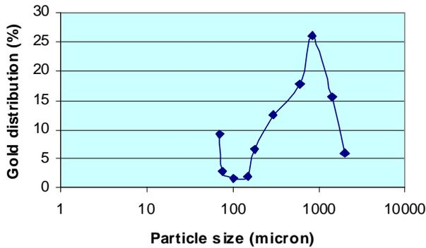
Figure 4. Distribution of gold particles in different sieve fractions.
