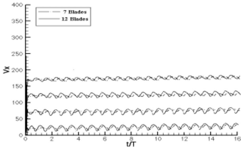
**Figure 10.** Comparison of velocity traces of 7 (dash dot lines) and 12 (solid lines) blades.
