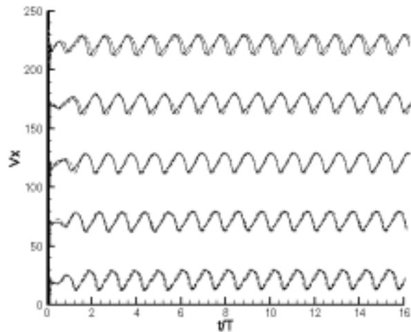
**Figure 9.** Comparison of velocity traces for 10 (dashed lines) and 14 (solid lines) blades.
