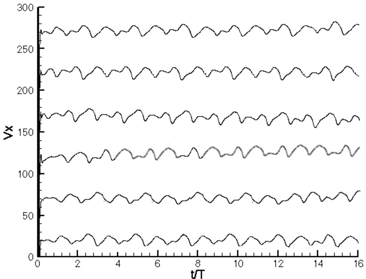
Figure 12. The velocity traces for 11-blade geometry at unstable condition.
