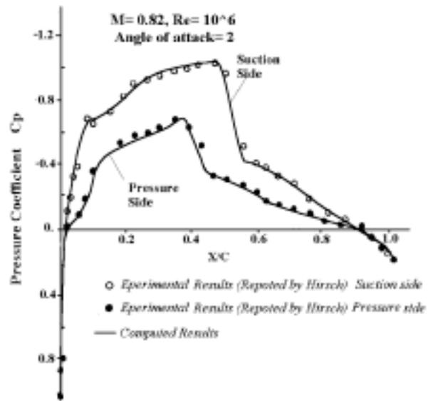
Figure 2. Computed and experimental pressure coefficients over a semi NACA0012 airfoil. Mach number is 0.82, the Reynolds Number is  $10^6$ , and at an angle of attack  $2^\circ$ .
