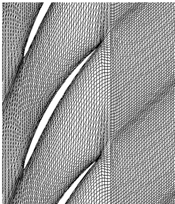
**Figure 5.** The sample enlarged mesh generated for rotor-cascade studies.
