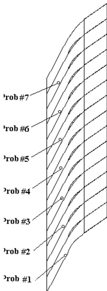
**Figure 4.** The 14-blade geometry and the location of the probes.
