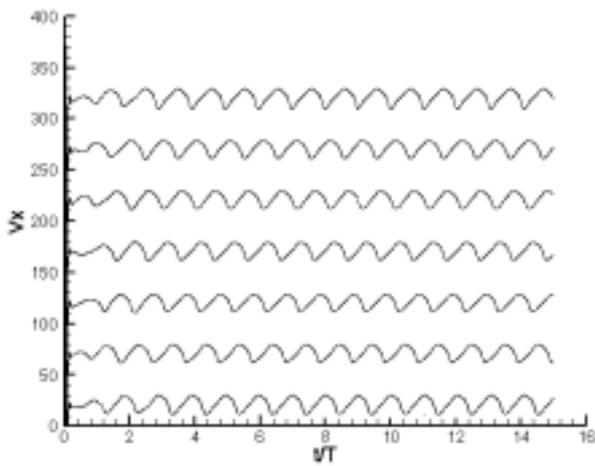
**Figure 6.** Velocity traces for 14-Blade geometry. The traces are shifted with constant interval for clarity.
