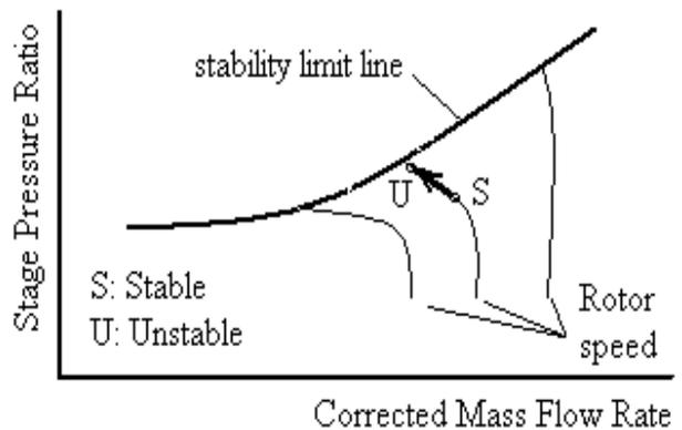
**Figure 3.** The thermodynamic path for reaching to RS condition from the normal operating point.
