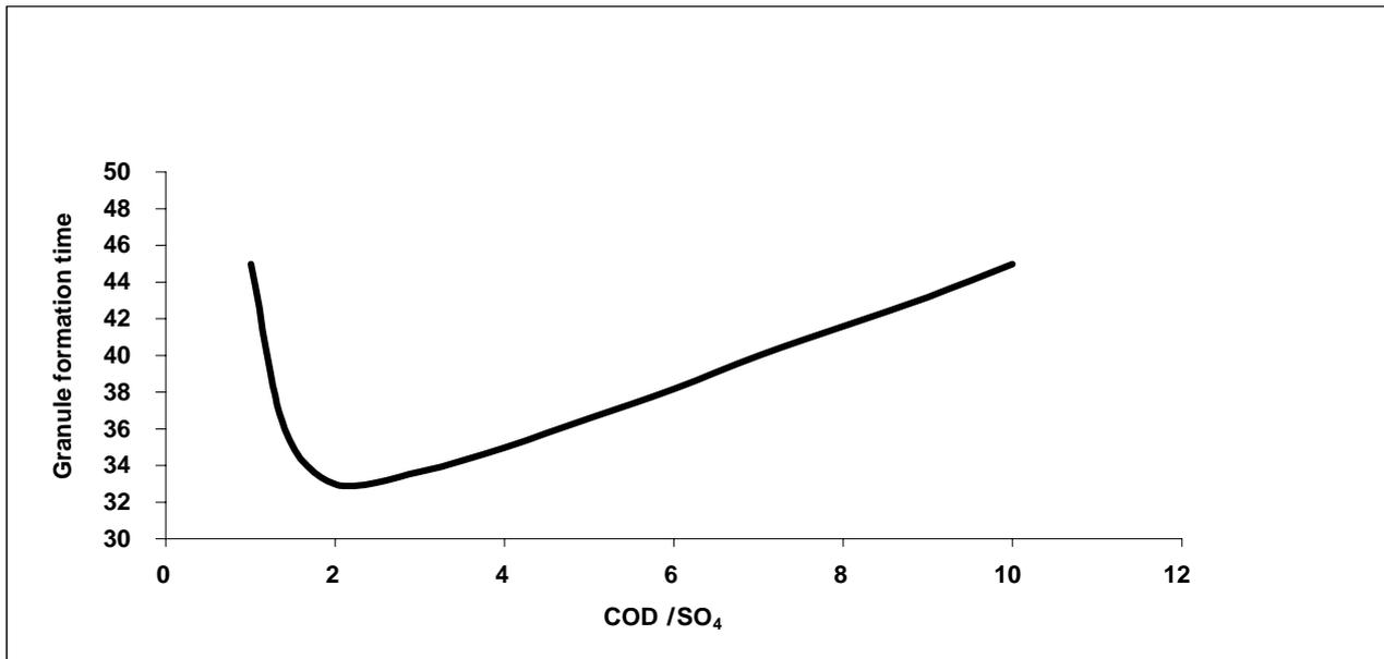
**Figure 4.** Effect of COD/SO<sub>4</sub> on granule formation time at COD=1000mg/l.
