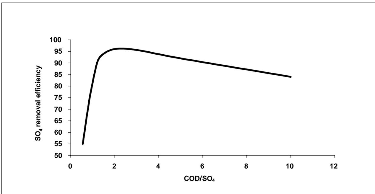
**Figure 3.** Effect of COD/SO<sub>4</sub> on SO<sub>4</sub> removal efficiency.
