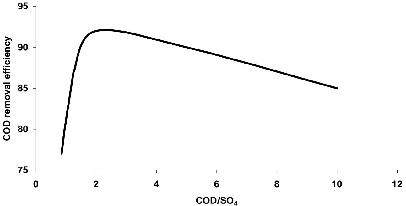
**Figure 2.** Effect of COD/SO<sub>4</sub> ratio on COD removal efficiency.
