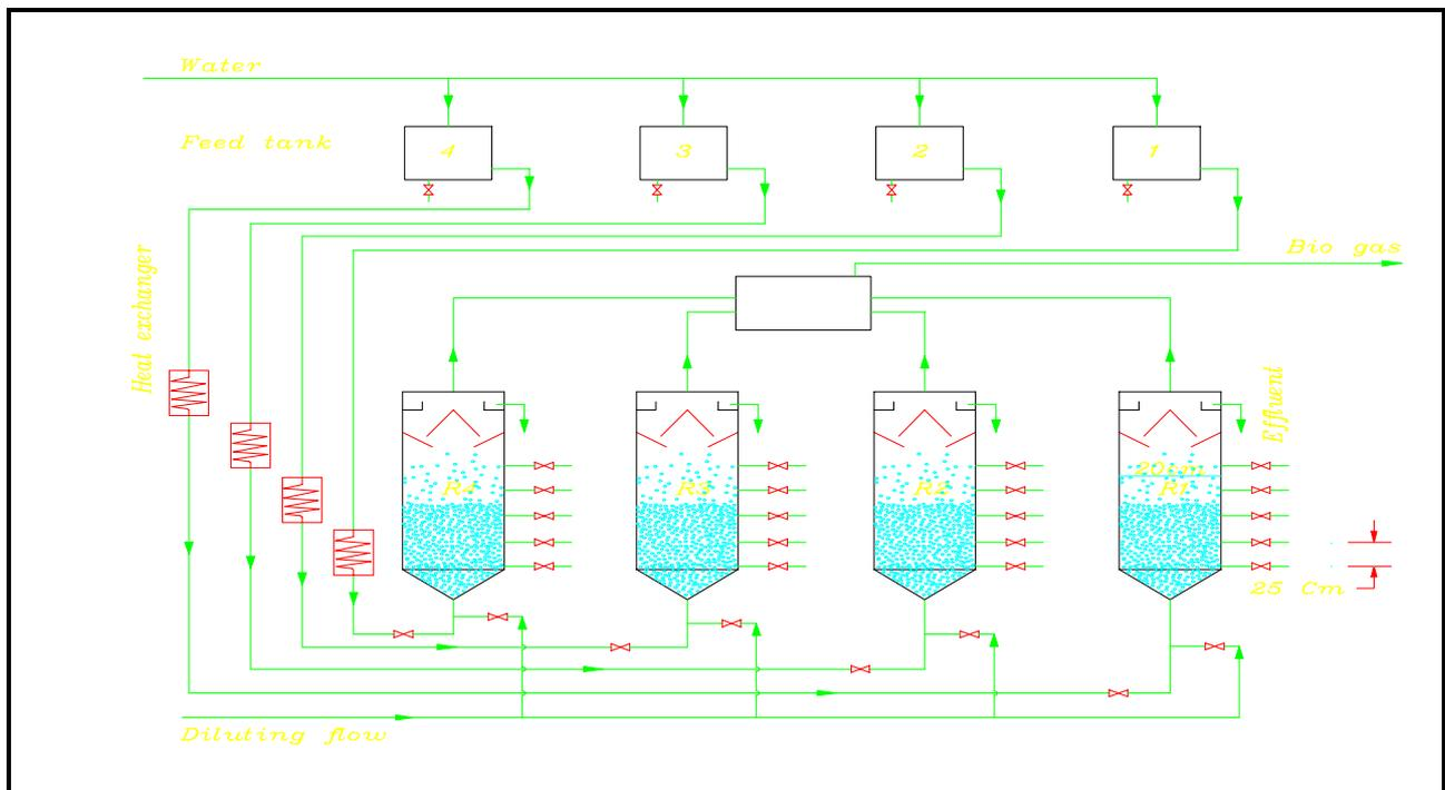
Figure 1. Schematic diagram for four pilots.
