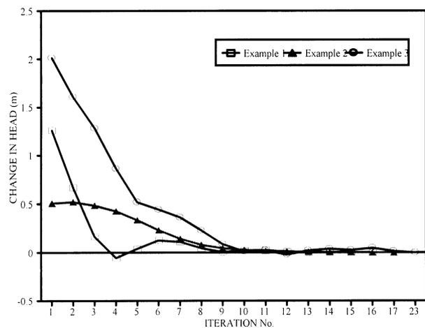
**Figure 6.** Changes in available head at Critical Nodes for Examples 1-3 using HDSM.
