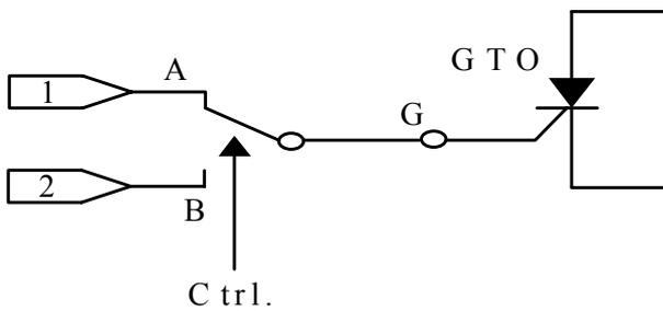
Figure 3. A simple ON/OFF controller usable in PSCAD/EMTDC simulated circuits.
