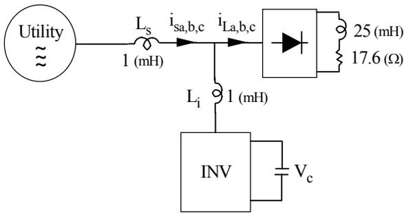
Figure 2. One line diagram of simulated power circuit.
