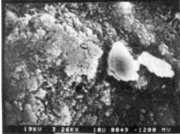
Figure 7. The dissolution of calcium hydroxide and formation of secondary gypsum.
