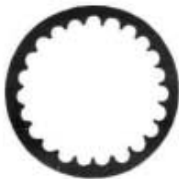
Figure 1. Cross section of ribletted pipe.
