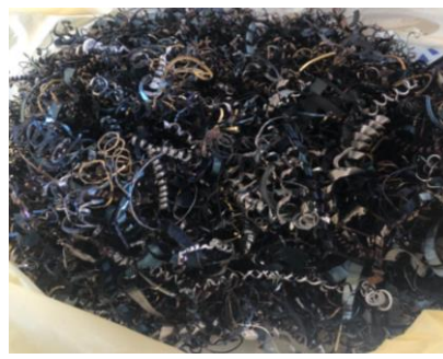
(b) Waste steel fibers after cutting
