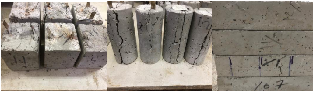
Figure 12. Concrete specimens after failure
