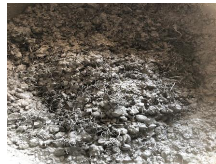
(c) The use of waste steel fibers in concrete
