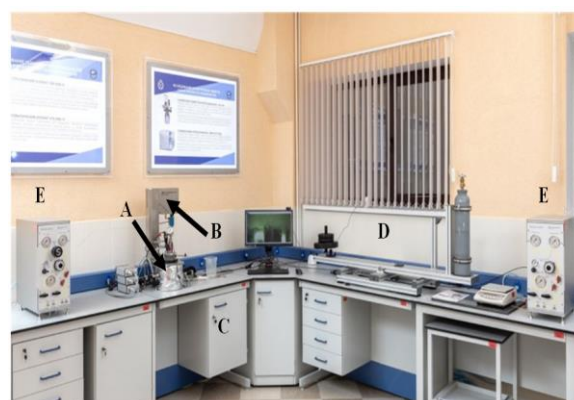
Figure 8. Laboratory complex for gas hydrate research: A. Autoclave GHA-350; B. Top-driven stirrer; C. Huber Ministat 240 thermostat; D. Gas boosters with maximum pressures of 40.0 MPa (left) and 15.0 MPa (right); E. Model gas preparation system.
