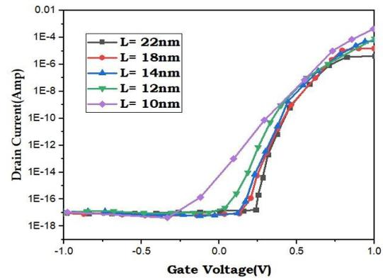
**Figure 5.** Drain current with gate voltage of proposed device at doping concentration  $N_d = 1 \times 10^{18} \text{ cm}^{-3}$
