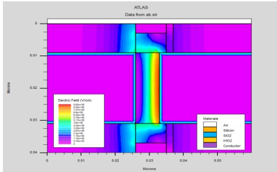
Figure 3. Electric field distribution of proposed device
