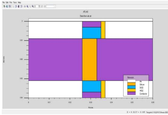
Figure 1. 2 D cross-sectional view of proposed Dual Material Gate Overlap on Drain Side TFET with spacer
