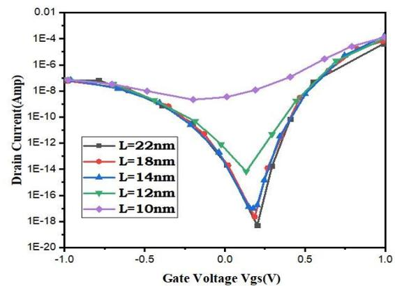
**Figure 6.** Drain current with gate voltage of proposed device at doping concentration  $N_d = 2 \times 10^{18} \text{ cm}^{-3}$
