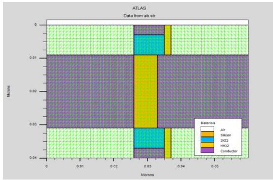
Figure 2. Mesh View of proposed device
