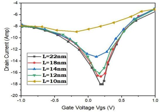
**Figure 7.** Drain current with a gate voltage of proposed device at doping concentration  $N_d = 3 \times 10^{18} \text{ cm}^{-3}$
