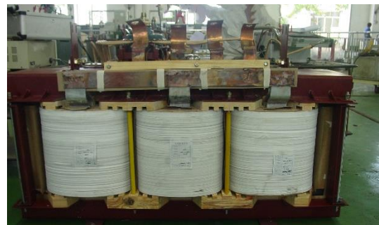
Figure 3. Model of a three-phase 1600kVA-22/0.4kV
