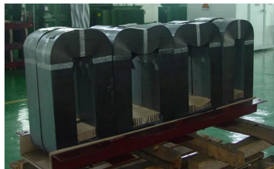
Figure 11. Steel core of the three-phase amorphous core transformer
