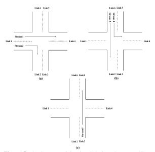
**Figure 5.** The Streams of the signal timing plan controlling the intersection (a) The Streams of Link 1 (b) The Streams of Link 6 (c) The Streams of Link 3
