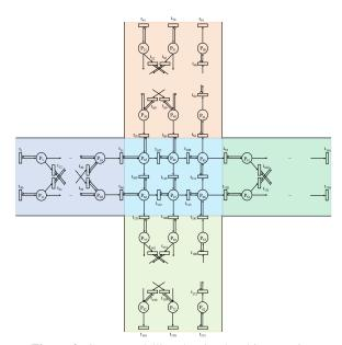
Figure 2. CTPN modelling the simulated intersection
