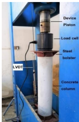
Figure 5. Test setup and instrumentation
