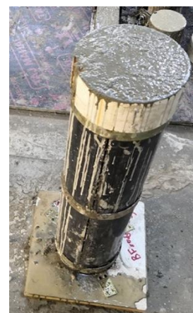
Figure 4. Concrete pouring into a mold
