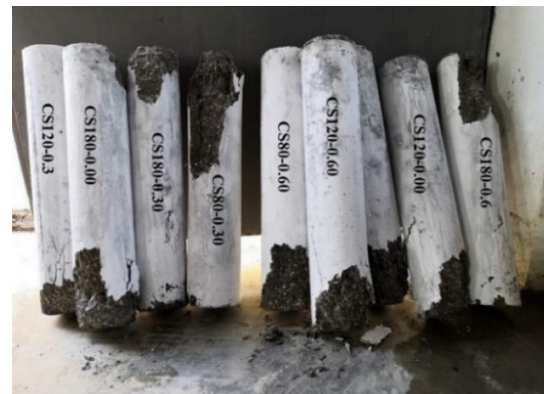
Figure 10. Failure patterns of short columns
