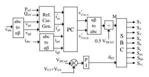
Figure 7. Grid-Tied IHTQZSC with CSF-PC
