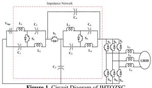
Figure 1. Circuit Diagram of IHTQZSC
