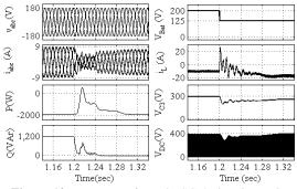
Figure 12. Response of IHTQZSC during QII to QI
