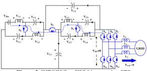
Figure 3. IHTQZSC as PWM inverter in nSTS
