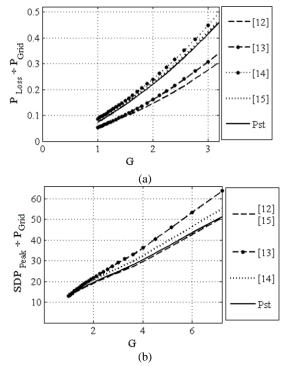
**Figure 6.** (a) Power loss variation with G (b) SDP variation with G
