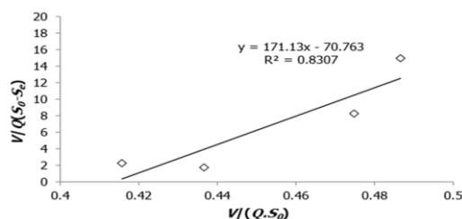
**Figure 6.** Plots of substrate removal for COD removal at HRT 12 h
