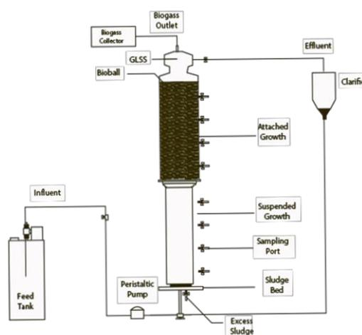
**Figure 1.** Schematic diagram of the Hybrid UASB reactor
