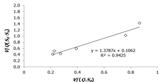
**Figure 5.** Plots of substrate removal for COD removal at HRT 18 h
