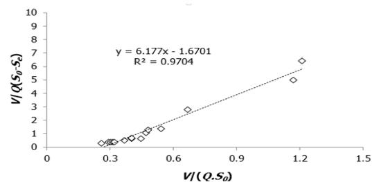
**Figure 4.** Plots of substrate removal for COD removal at HRT 24 h
