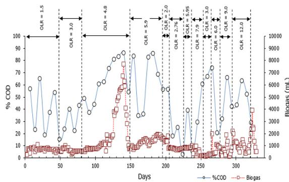
**Figure 2.** Relationship between % COD and biogas on OLRs
