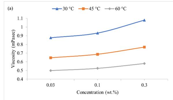
**Figure 3(a).** Variation of viscosity with concentration
