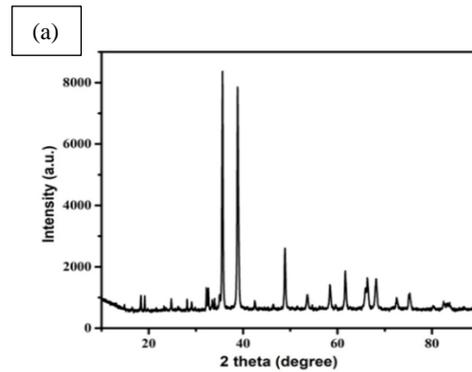
Figure 1(a). XRD pattern of CuO nanoparticles
