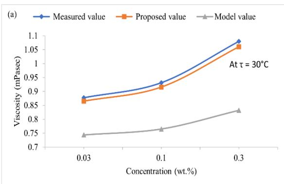
Figure 6 (a). Viscosity versus concentration at 30°C
