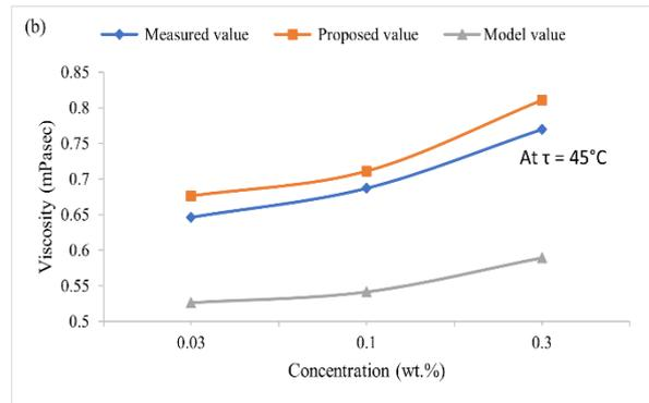
Figure 6 (b). Viscosity versus concentration at 45°C
