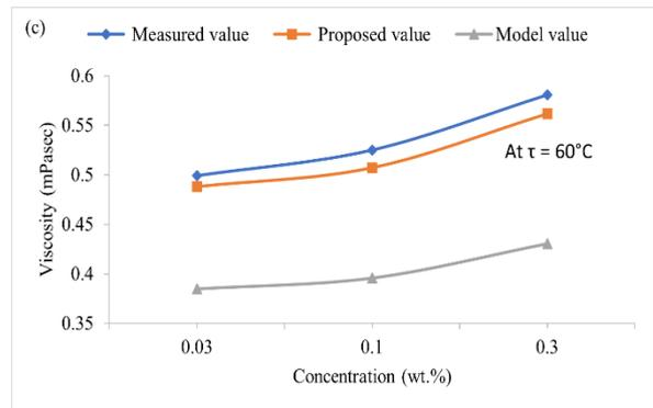
Figure 6(c). Viscosity versus concentration at 60°C
