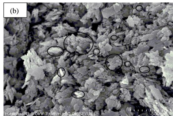
Figure 2(b). FESEM image of CuO nanoparticles
