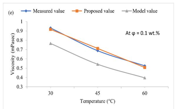
Figure 6(e). Viscosity versus temperature at 0.1 wt.%
