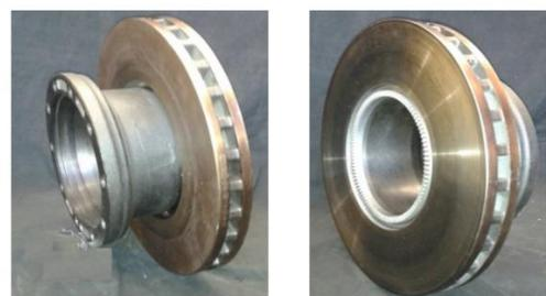
**Figure 2.** Brake disc analysed: a) Outboard view; b) Inboard view
