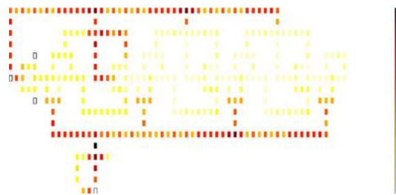
Figure 17. Energy diagram of proposed 4-bit testable shift register
