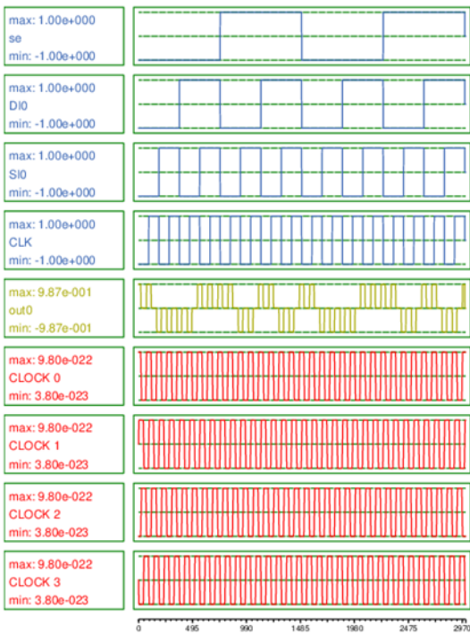
Figure 16. simulation result of scan cell
