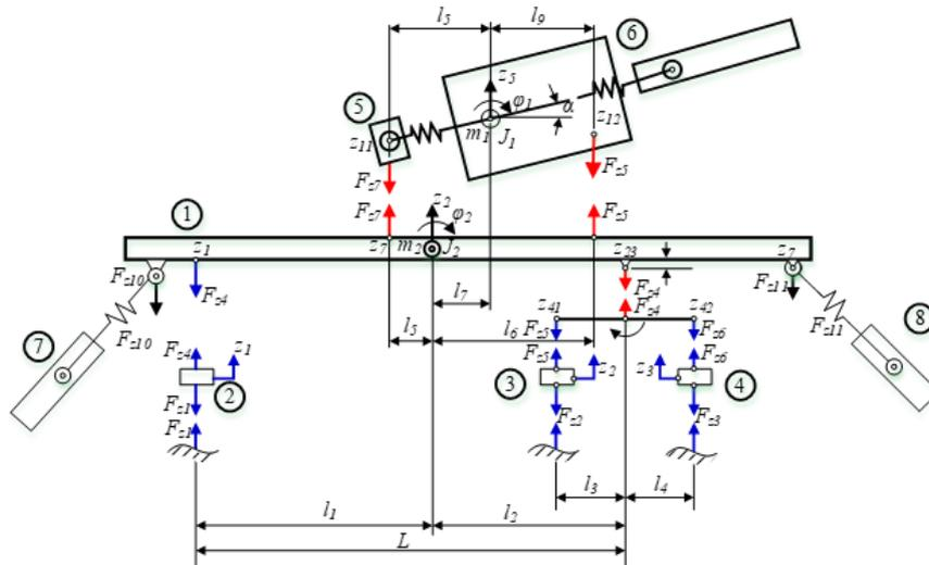
**Figure 3.** Multi-purpose forest fire fighting vehicle model: 1. Chassis of the vehicle; 2. Front axle; 3. Middle axle; 4. Rear axle; 5. Water pump for fire fighting; 6. Fire sprinkler; 7. Tree cutting structure creates a white corridor; 8. Lawn cleaning machine clears the way
