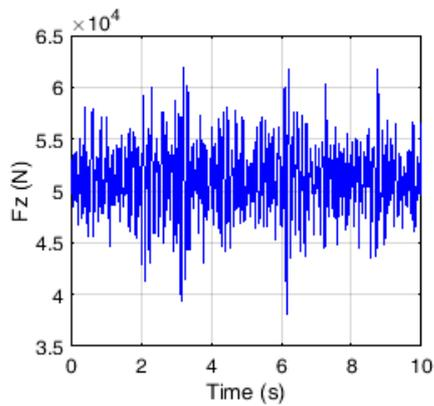
**Figure 17.** Dynamic load acting on the chassis at the rear axle,  $v = 15 \text{ km/h}$ ,  $C_4 = 401952 \text{ N/m}$ ,  $C_{5,6} = 527042 \text{ N/m}$
