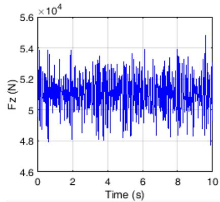
Figure 14. Dynamic load acting on the chassis at the rear axle,  $v = 10 \text{ km/h}$ ,  $C_4 = 203000 \text{ N/m}$ ,  $C_{5,6} = 322000 \text{ N/m}$
