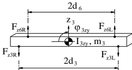
Figure 8. Object separation model of rear axle
