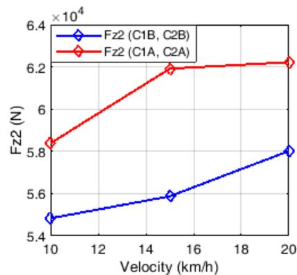
**Figure 21.** Maximum dynamic load acting on the chassis rear axle,  $v = 10 \div 20 \text{ km/h}$
