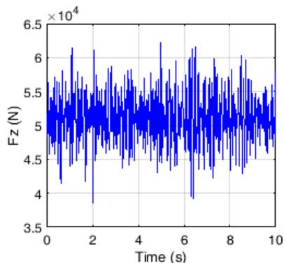
**Figure 19.** Dynamic load acting on the chassis at the rear axle,  $v = 20 \text{ km/h}$ ,  $C_4 = 401952 \text{ N/m}$ ,  $C_{5,6} = 527042 \text{ N/m}$
