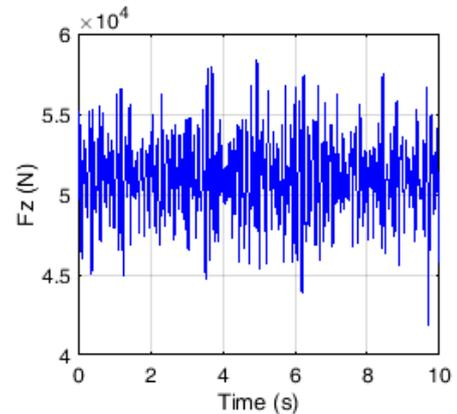
Figure 15. Dynamic load acting on the chassis at the rear axle,  $v = 10 \text{ km/h}$ ,  $C_4 = 401952 \text{ N/m}$ ,  $C_{5,6} = 527042 \text{ N/m}$
