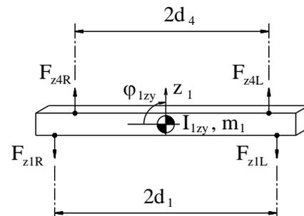
**Figure 4.** Object separation model of front axle
