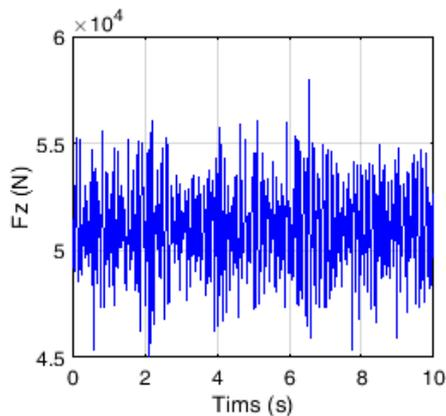
**Figure 18.** Dynamic load acting on the chassis at the rear axle,  $v = 20 \text{ km/h}$ ,  $C_4 = 203000 \text{ N/m}$ ,  $C_{5,6} = 322000 \text{ N/m}$
