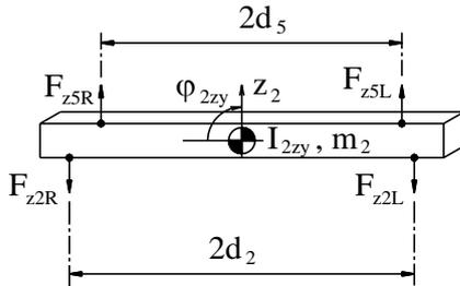
Figure 6. Object separation model of middle axle
