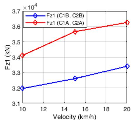
**Figure 20.** Maximum dynamic load acting on the chassis front axle,  $v = 10 \div 20 \text{ km/h}$
