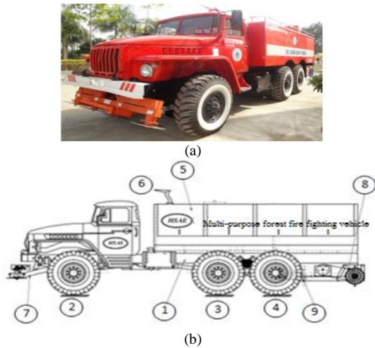
**Figure 1.** (a) Multi-purpose forest fire fighting vehicle (b) Overall multi-purpose forest fire fighting vehicle: 1. Vehicle, 2. front drive axle, 3. middle drive axle, 4. rear drive axle, 5. Water pump equipment, fire water tank, 6. water nozzle, 7. Equipment to cut trees, clean garbage, pave the way to create a fire isolation corridor, 8. Equipment to clean grass on the road, 9. Fire-fighting sandblasting equipment [1-3,5]
