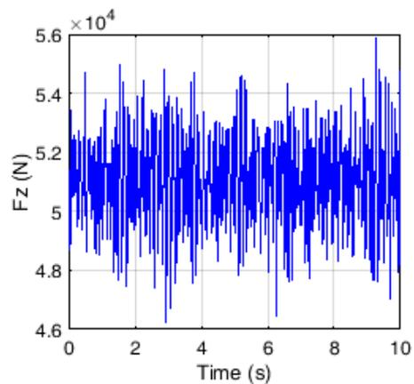
Figure 16. Dynamic load acting on the chassis at the rear axle,  $v = 15 \text{ km/h}$ ,  $C_4 = 203000 \text{ N/m}$ ,  $C_{5,6} = 322000 \text{ N/m}$
