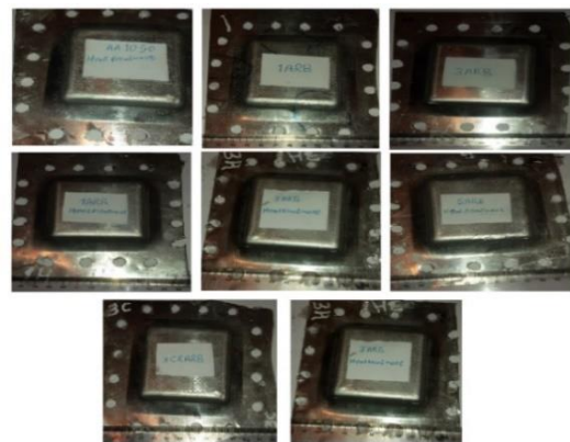
Fig. 9: Samples produced by experimental SPIF processes
