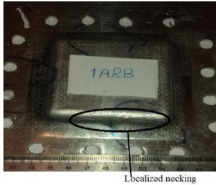
Fig. 10: Onset of localized necking
