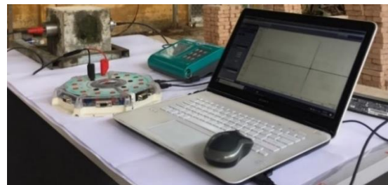
Figure 7. Device connection diagram to receive wave signal
