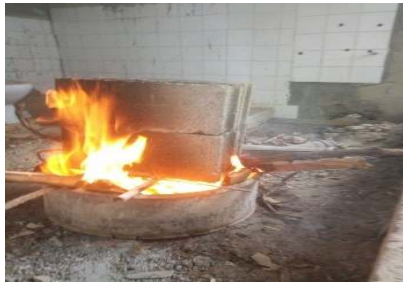
Figure 5. Fire resistance test
