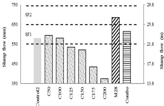
Figure 9. Results of J-ring test
