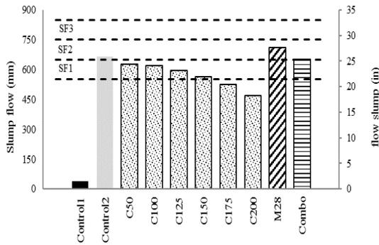
Figure 7. Results of slump flow test
