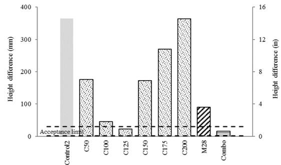
Figure 14. Results of U-Box test
