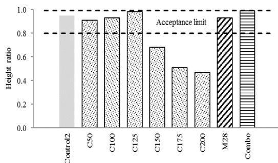
Figure 13. Results of L-Box test
