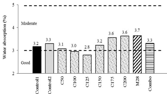
**Figure 17.** Results of water absorption test
