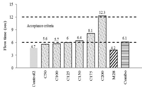
Figure 11. Results of V-funnel test
