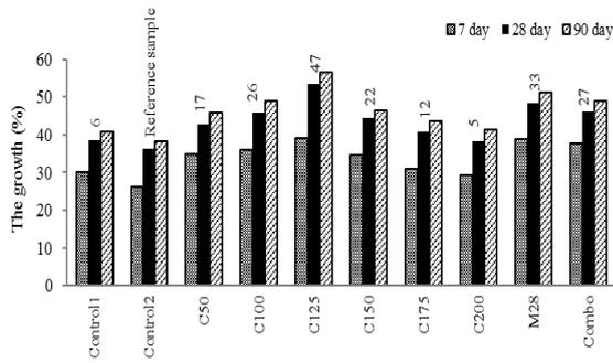
**Figure 16.** Compressive strength growth of samples at the different ages in comparison to control sample 2
