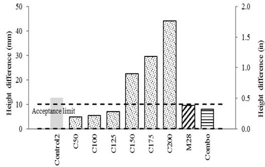
Figure 10. Height difference between the slump flow inside and outside of the J-ring
