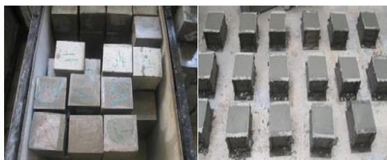
**Figure 5.** Preparation of concrete blocks
