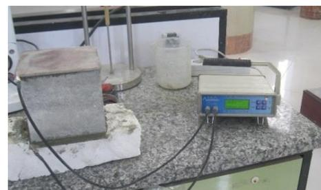
**Figure 6.** Electrical resistivity apparatus
