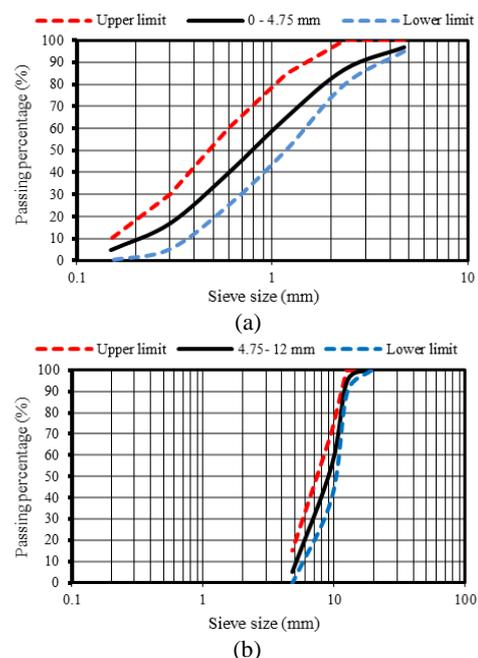
**Figure 1.** Gradation curves for aggregates: (a): sand aggregate, (b): gravel aggregate
