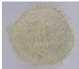
**Figure 2.** Image of calcium carbonate powder used in mix design
