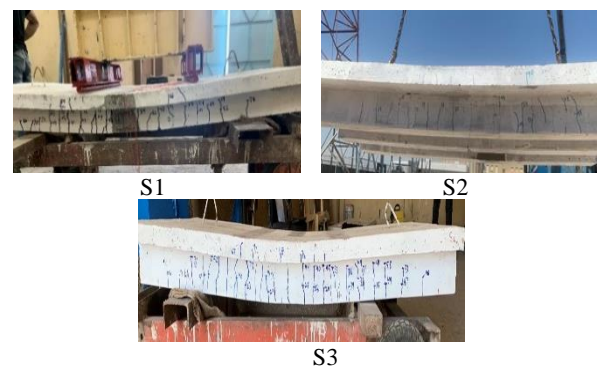
Figure 4. Cracking patterns for specimens tested under static load
