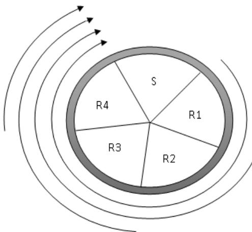
Figure 1. Repair technique on the same welding joint (Repair sequences).
