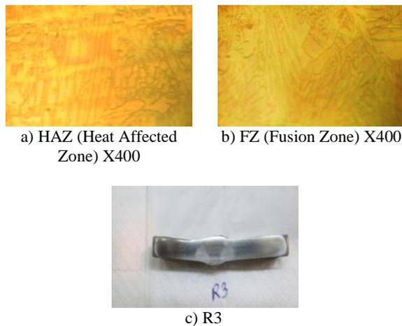
**Figure 10.** Micrographs after the third repair
