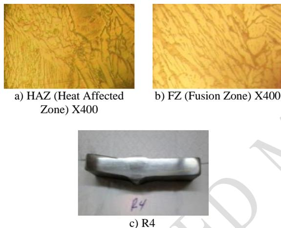
**Figure 11.** Micrographs after fourth repairs
