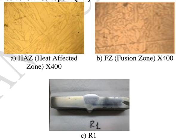
Figure 8. Micrographs after the first repair
