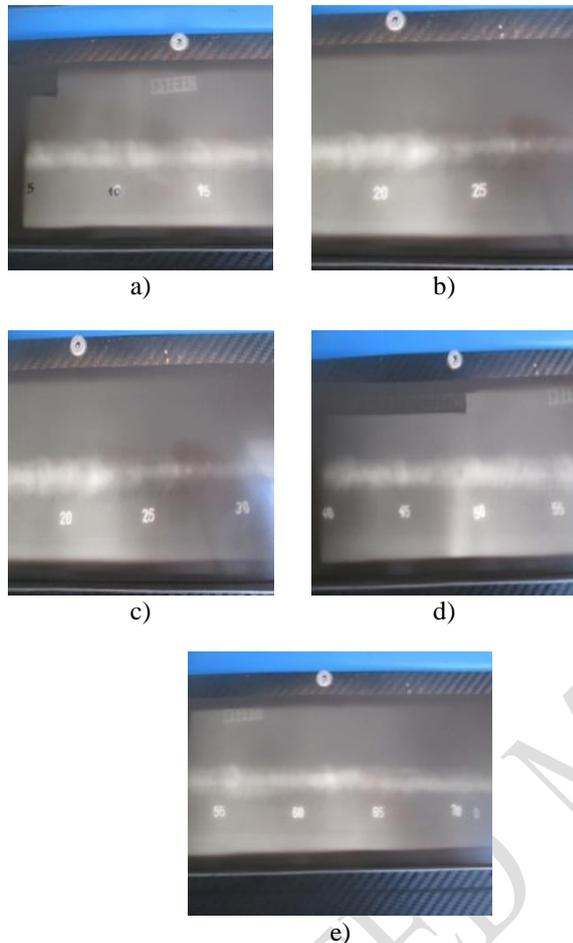
Figure 6. Radiographic stereotypes after repairs
