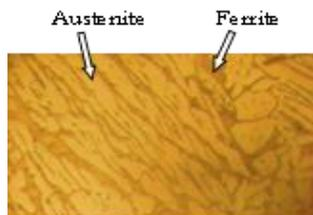
**Figure 12.** Ferrite dark and austenite light 400X
