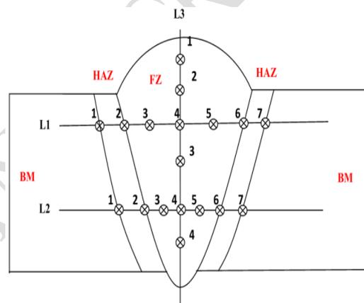
**Figure 3.** Hardness points measurements
