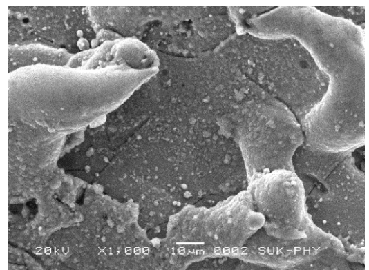
Figure 7. Micro-cracks of machined surface
