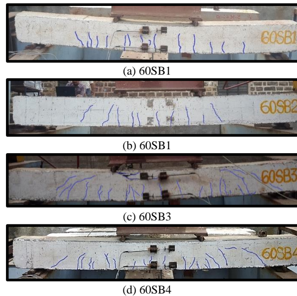
Figure 12. Crack pattern and failure modes for M 60 grade
