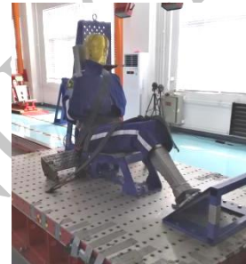
Figure 3. R16 dummy restrained by a 3-point seat belt on the trolley of acceleration type
