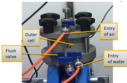
Plate 1. The modified Oedometer cell.
