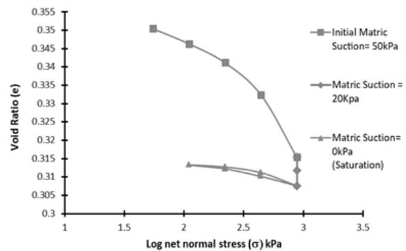
**Figure 6.** The void ratio versus log net normal stress for different matric suction under stress level of 885 kPa.
