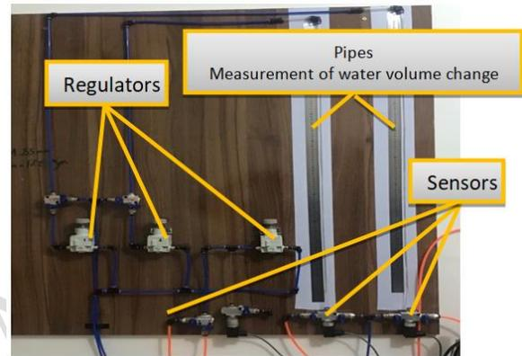
Plate 2. The control board
