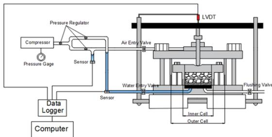
Figure 3. The scheme of the used tools and equipment.
