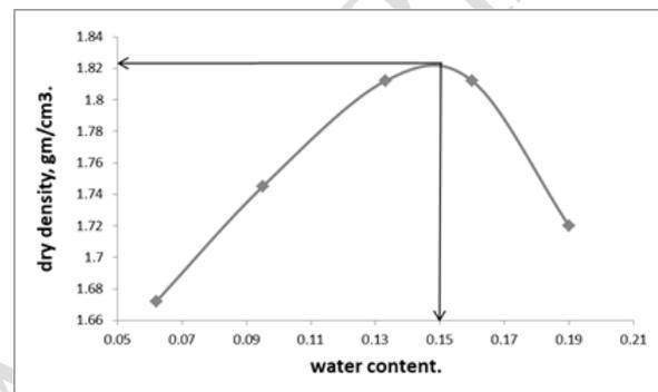
Figure 2: The results of standard Proctor test.
