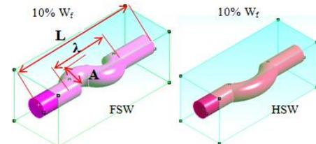
**Figure 4.** Finite Element models with fiber waviness
