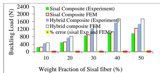
**Figure 8.** Buckling load from Experimental and FE results with percentage error
