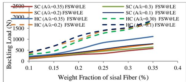
Figure 13. Buckling load of FSW at the Load end
