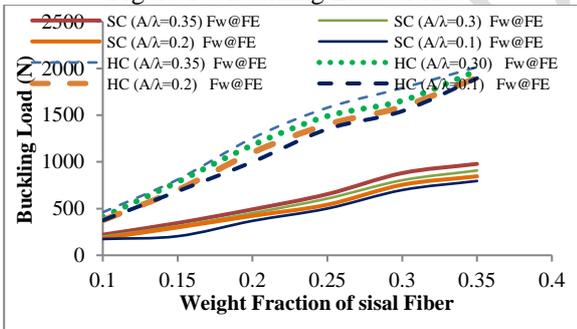
Figure 11. Buckling load of FSW at the fixed end
