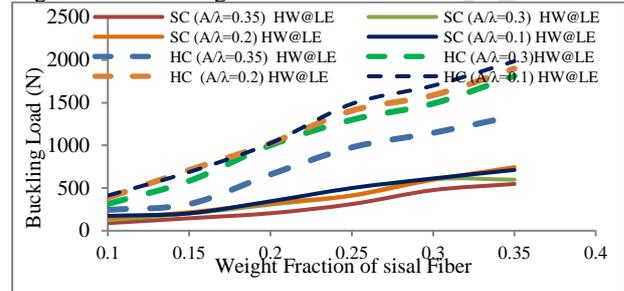
Figure 14. Buckling load of HSW at the Load end
