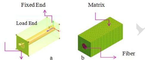
**Figure 3.** FE model and Finite element mesh
