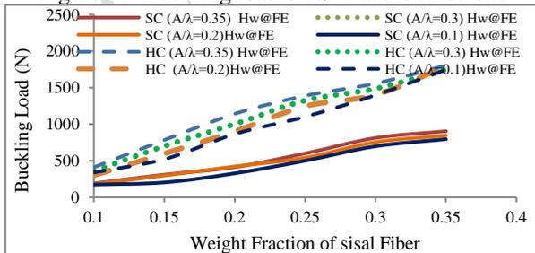
Figure 12. Buckling load of HSW at the fixed end
