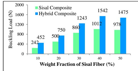
**Figure 7.** Buckling Load of sisal and Hybrid composites
