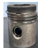
Figure 2. Coated piston after testing
