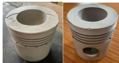
Figure 1. Uncoated and Coated Piston before testing
