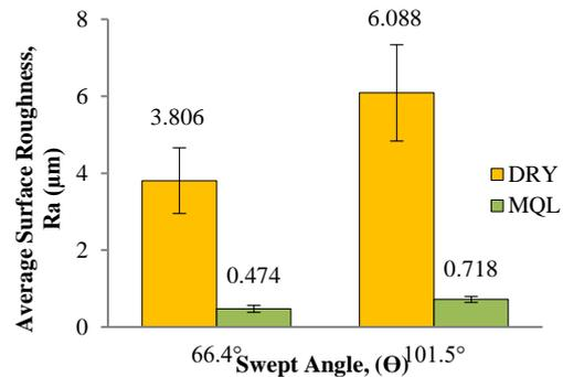
**Figure 7.** Average comparisons for surface roughness,  $R_a$ .
