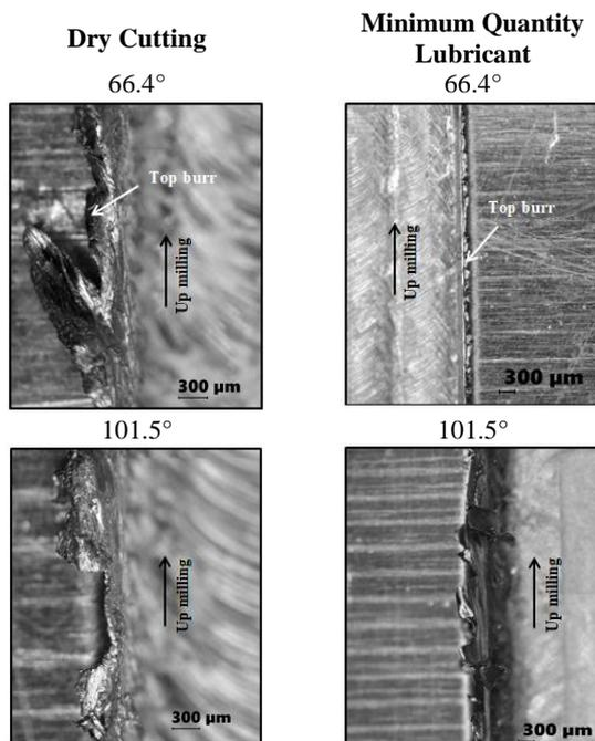
**Figure 9.** Burr formation under different swept angles and cutting conditions
