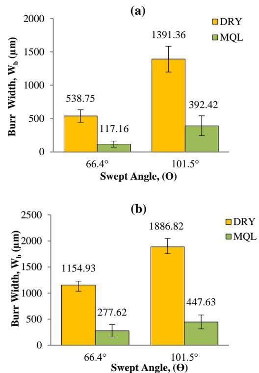
**Figure 10.** Average burr width under different cutting condition after (a) 1<sup>st</sup> slot; and (b) 10<sup>th</sup> slot
