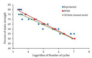
**Figure 6.** Comparison between fatigue life prediction of [30]<sub>16</sub> laminate from different numerical models
