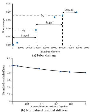
Figure 2. Longitudinal direction damage
