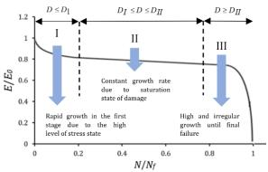
Figure 1. Overall stiffness reduction in fatigue loading
