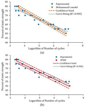
**Figure 7.** Fatigue life simulation and experimental results of [30]<sub>16</sub> laminate
