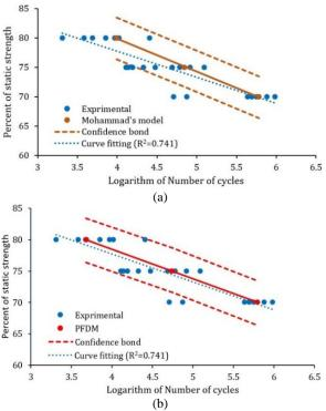
**Figure 8.** Fatigue life simulation and experimental results of [90/45/-45/0]<sub>s</sub> laminate
