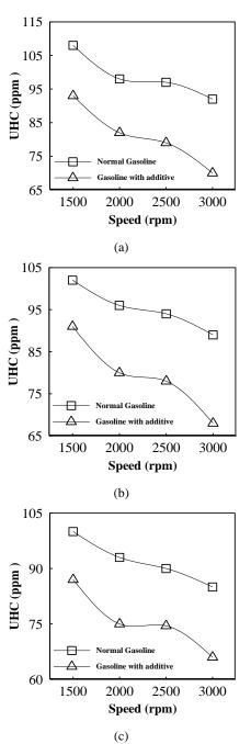
**Figure 10.** Experimental results of unburned hydrocarbons for (a) Engine with single electrode spark plug, (b) Engine with dual electrode spark plug, (c) Engine with platinum+4 spark plug at different fuel blends and engine speeds
