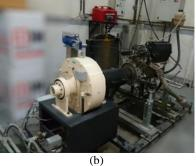
Figure 1. View of (a) the dynamometer and (b) the engine test bed
