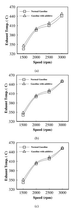
**Figure 11.** Experimental results of temperature of the exhaust gases for (a) Engine with single electrode spark plug, (b) Engine with dual electrode spark plug, (c) Engine with platinum+4 spark plug at different fuel blends and engine speeds
