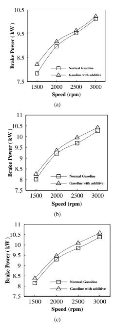
**Figure 5.** Experimental results of brake power for (a) Engine with single electrode spark plug, (b) Engine with dual electrode spark plug, (c) Engine with platinum+4 spark plug at different fuel blends and engine speeds
