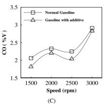
**Figure 8.** Experimental results of carbon monoxide for (a) Engine with single electrode spark plug, (b) Engine with dual electrode spark plug, (c) Engine with platinum+4 spark plug at different fuel blends and engine speeds
