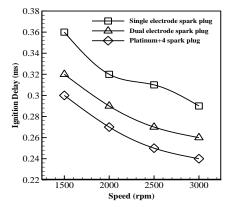
**Figure 7.** Variations of ignition delay according to different engine speeds for different types of spark plugs using pure gasoline
