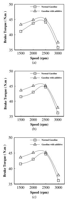
**Figure 4.** Experimental results of brake torque for (a) Engine with single electrode spark plug, (b) Engine with dual electrode spark plug, (c) Engine with platinum+4 spark plug at different fuel blends and engine speeds
