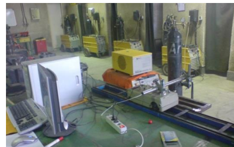
Figure 1. Mechanical components of the automatic arm of the gas tungsten arc welding
