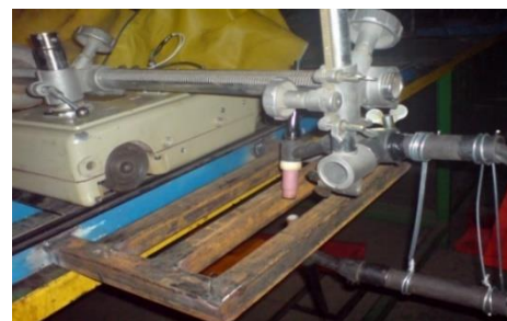
Figure 3. Double-sided torch to further protect argon from subsamples
