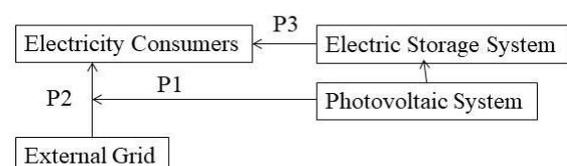
Figure 1. The generalized power supply system block diagram
