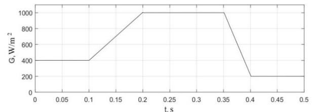
**Figure 3.** The changes of the solar radiation intensity
