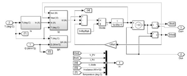
Figure 6. Internal structure of the PV Array subsystem
