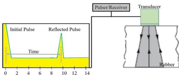
Figure 1. Schematic of Ultrasonic Test
