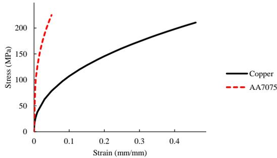
Figure 4. The stress-strain diagram of AA7075 and copper [22,23]
