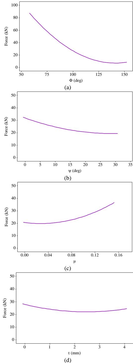
**Figure 6.** Main effect of a)  $\Phi$ , b)  $\Psi$ , c)  $\mu$ , and d)  $t$  on the maximum force
