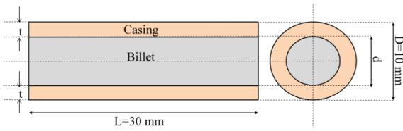
Figure 3. Schematic geometry and dimensions of samples
