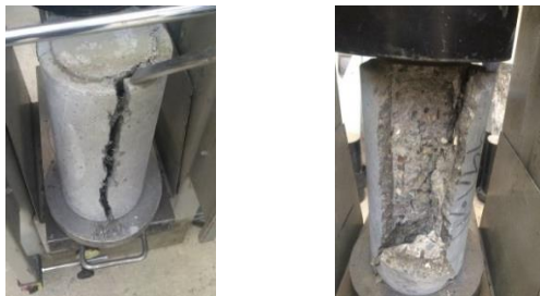
Figure 4. Cracking pattern of repaired specimens in patch tests
