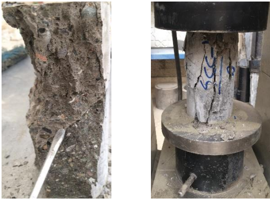
Figure 7. Failure pattern of typical specimens in slant shear tests
