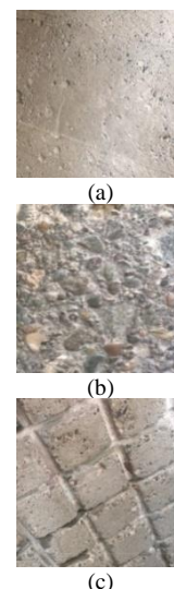
Figure 3. Surface preparations in slant shear tests, a) smooth surface, b) brushed surface, c) grooved surface
