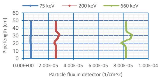
**Figure 4.** Photon log for various photon energies along the pipe with CaCO<sub>3</sub> deposition (deposition thickness is equal to 20% of internal pipe diameter and deposition length is equal to 1 cm)
