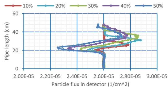
**Figure 7.** Photon log for various deposition thicknesses of CaCO<sub>3</sub> (deposition thickness=10, 20, 30, 40, and 50% of internal pipe diameter, deposition length=1 cm, photon energy=200 keV)
