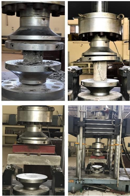
Figure 2. 1000kN servo-controlled test setup
