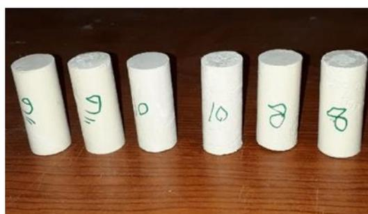
**Figure 1.** Geopolymer cement paste specimen
