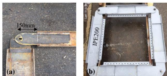
Figure 2. The frame setup: a) beam to column connection and b) the frame assembly
