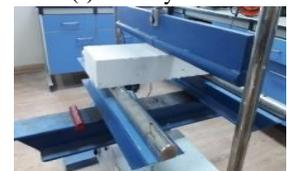
(e) Modulus of rupture test
