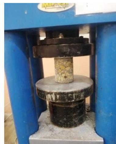
Figure 5. LWC cores under compression test
