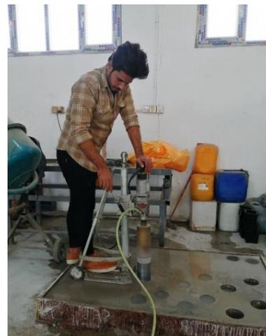
Figure 4. Concrete core drilling of LWC slab
