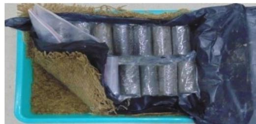
Figure 2. UCC samples under curing process
