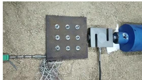
**Figure 7.** Horizontal load applied on model piled raft foundation
