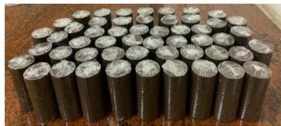
Figure 1. UCC samples in polyethene wrapper
